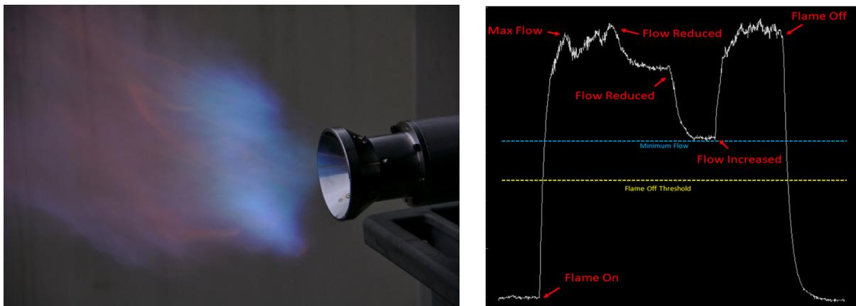
**Figure 3 (a) Proof of concept burner firing, (b) Example output measurements showing the capability of high-resolution measurement of ion concentrations within the flame.**
