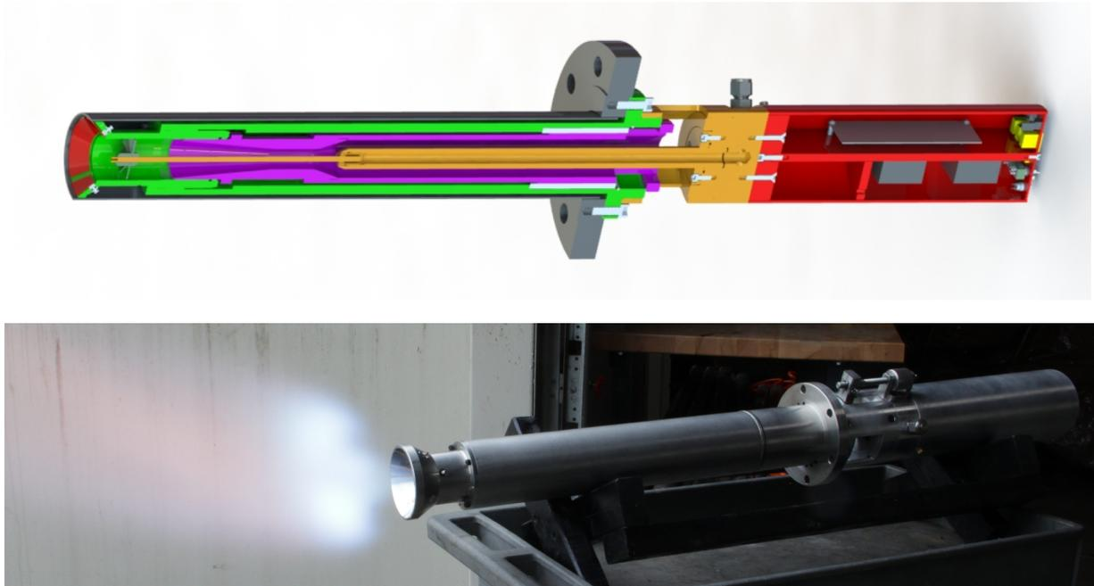
**Figure 2 Proof of concept burner with integrated flame detector**
