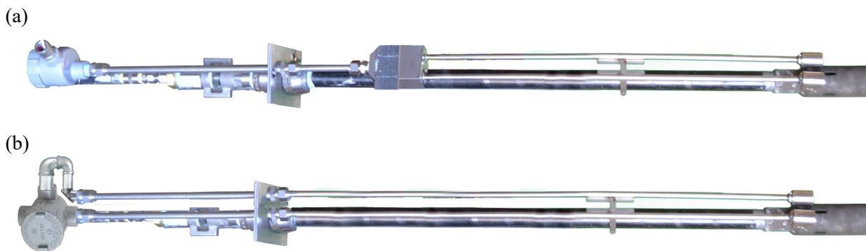
**Figure 4 Two configurations for the ClearSign EYE: (a) 2-to-1 probe configuration with single feedthrough on the pilot mounting plate, (b) 2-probe configuration with two feedthroughs on the pilot mounting plate**
