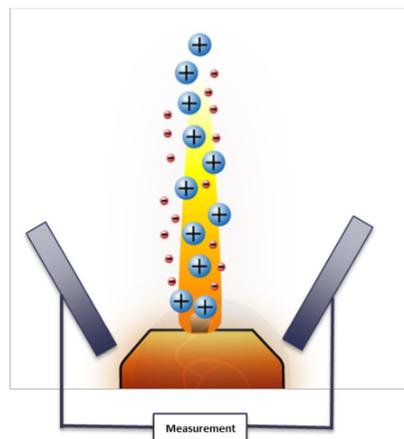
Figure 1 Flame detection using two capacitively coupled probes
